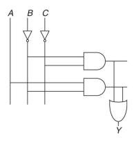
$$Y = \overline{A}\,\overline{B}\,\overline{C} + A\overline{B}\,\overline{C} + A\overline{B}C$$
