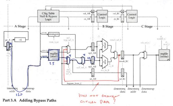
Add bypass paths to the datapath diagram to ensure it is "fully bypassed" meaning every reasonable bypass path is included.
