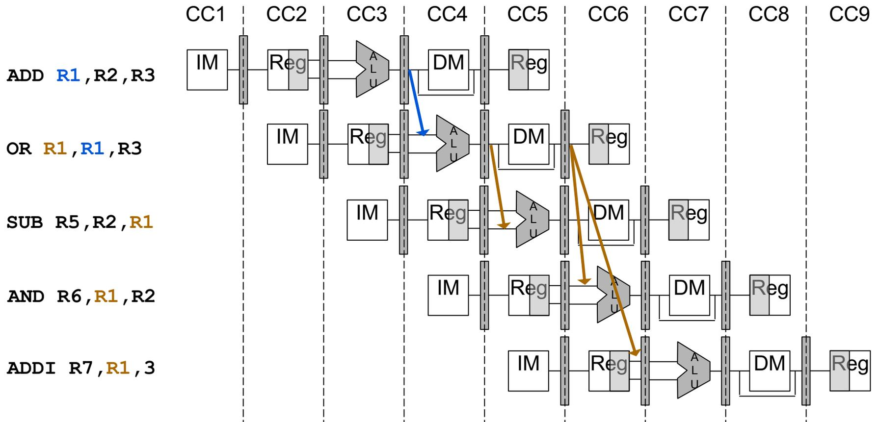
Forwarding path from **ADD** to **SUB** (via **WB→EX**) must be disabled so the updated R1 produced by **OR** is forwarded to **SUB** (via **MEM→EX**)
