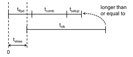
Given these conditions, the data signal still has to win the race, but because of clock skew, it does not have to run as quickly.
