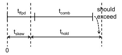
The following inequality should hold for the setup time constraint to be met:
