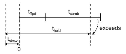
The following inequality should hold for the hold time constraint to be met:
