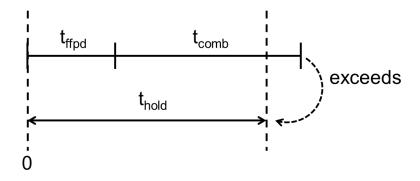
As shown in the above diagram, the sum of  $t_{ffpd}$  and  $t_{comb}$  has to be greater than  $t_{hold}$ . Otherwise, it would be as if the earlier member of the relay team (flip-flop A) did not give the later member (flip-flop B) enough time to grab on, and the baton was dropped.
