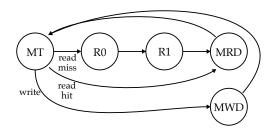
We will need to keep valid bits in the control unit, with one valid bit for every cache line. We will also need to keep use bits which are updated on every access to indicate which was the last "used" line. Assume we create the following two control signals generated by the FSM control unit.
