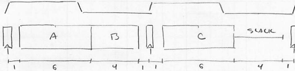
$$t_c = \max(t_{pcq} + t_{pd,A} + t_{pd,B} + t_{setup}, t_{pcq} + t_{pd,C} + t_{setup})$$
