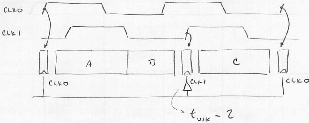
$$t_c = \max(t_{poq} + t_{pd,A} + t_{pd,B} + t_{setup} - t_{usk}, t_{usk} + t_{poq} + t_{pd,C} + t_{setup})$$
